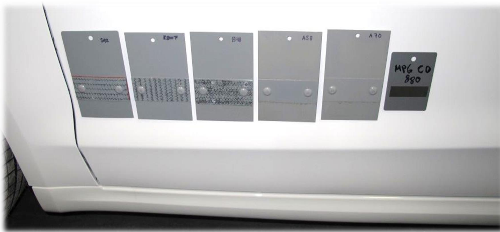
Coupons mounted to lower doors of a corrosion test vehicle, run for 12 weeks through full vehicle accelerated corrosion test
